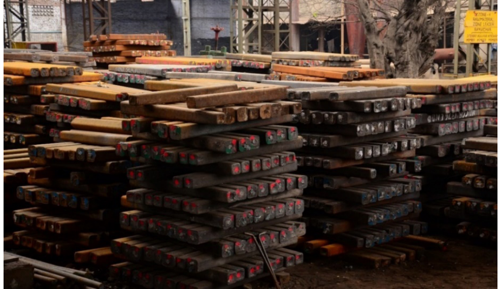
Figure 13: Billets formed from scrap steel
