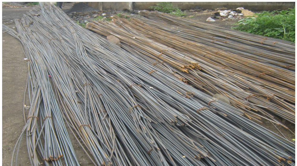
Figure 14: TMT bars produced from billets
